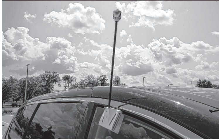
A sensor is seen July 22 on a volunteer's car as part of the "Spot the Hot" program in Cedar Rapids. The NOAA grant-funded program seeks to map heat islands using data collected by volunteers.
