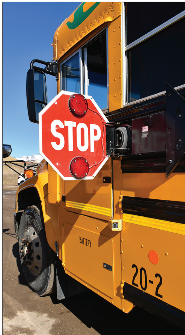
Drivers approaching a bus will see a stop sign like this, with the red lights engaged above the emergency exit on the back of the bus. Pictured is the recently installed camera below the extended sign.
