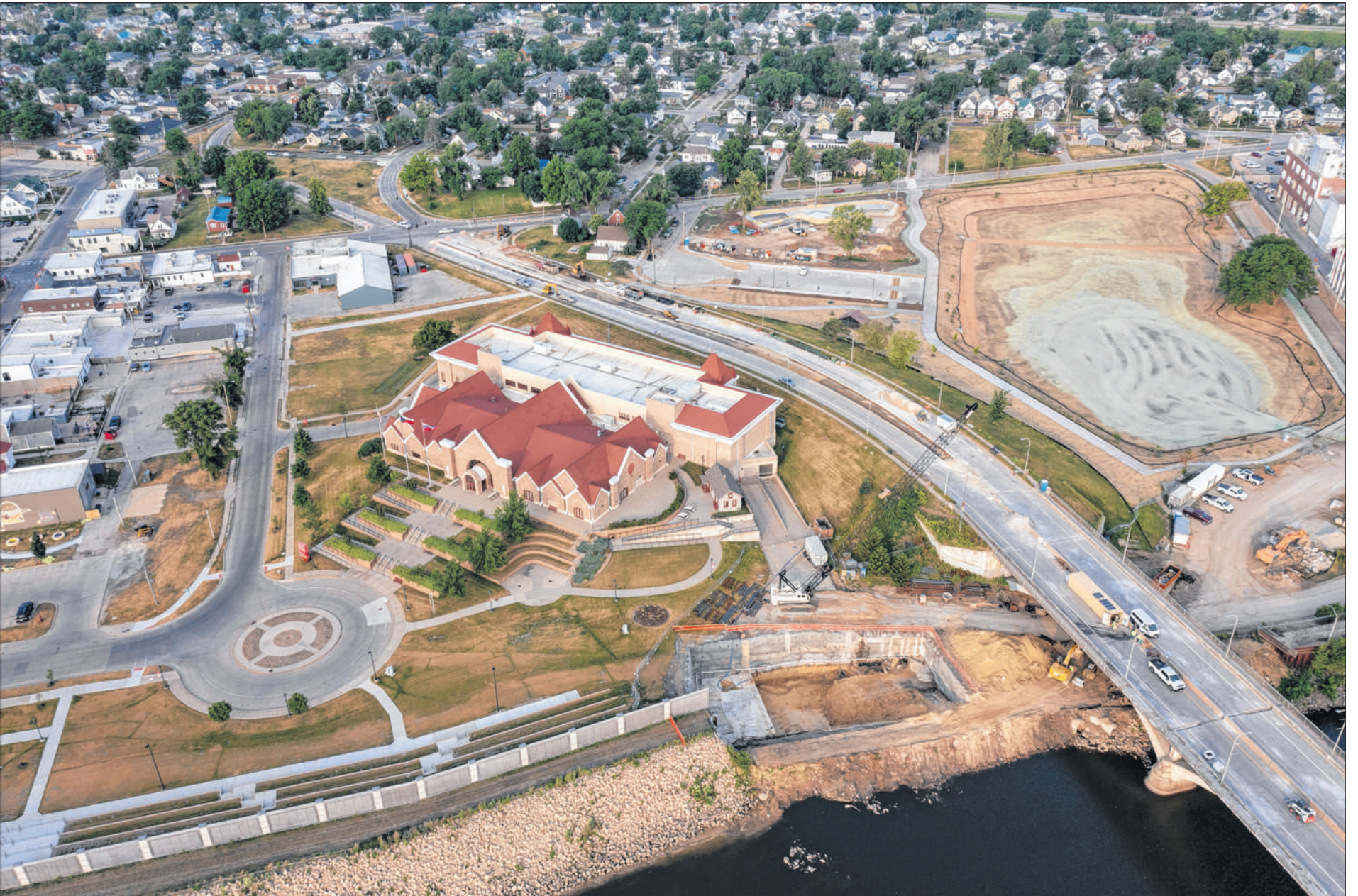
Flood control infrastructure surrounds the National Czech & Slovak Museum & Library in an aerial photo Thursday in southwest Cedar Rapids. Flood walls are visible in the bottom left, while the site of construction on flood control measures around the 12th Avenue Bridge and a retention basin in Riverside Park are also visible. (Nick Rohlman/The Gazette)
