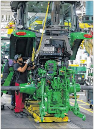
Julian Roby helps attach the cab to a John Deere tractor in 2016 at the Deere assembly plant in Waterloo. The company recently yielded to pressure from right-to-repair advocates, saying it will begin sharing information farmers need to fix their machines without involving a Deere-approved repair shop. (Brandon Pollock/ Waterloo-Cedar Falls Courier)
