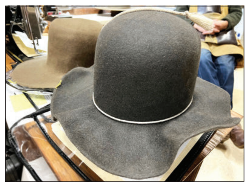
Gibson often uses felt to make hats. The felt comes to him in an un-sized bell shape and has to be blocked into a size and shape using moisture and steam. The hat making process also includes ironing, stiffening, sanding and cutting. It takes a combined eight hours over a roughly one-week period.
